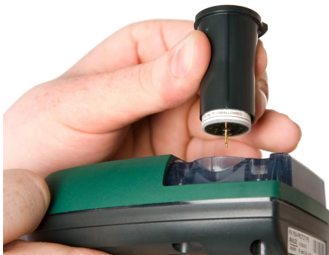
Figure 41 Align the new sensor with the ADM Aspida device
