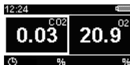
Figure 18 The main gas display showing that the user has exceeded their TWA exposure to carbon dioxide
