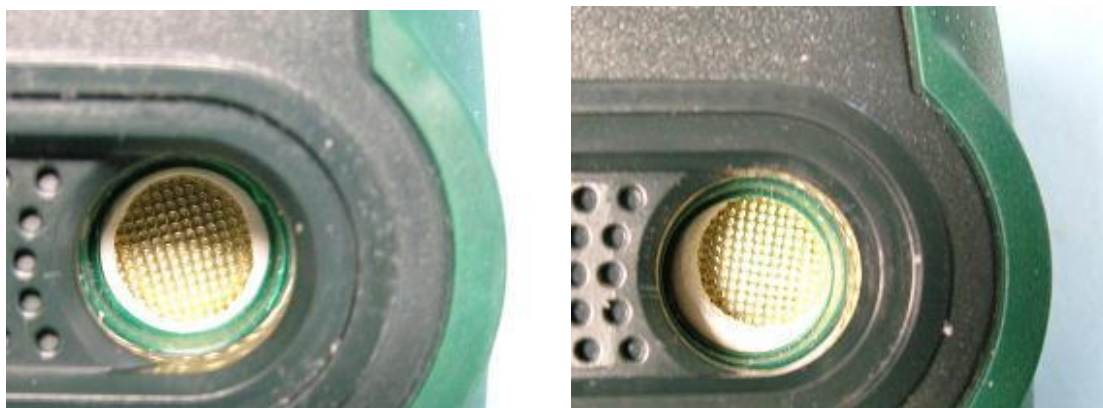
Figure 43 Centralised and misaligned sensors
