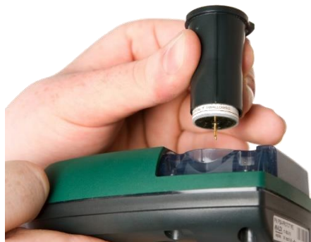
Figure 6 Align the new sensor with the ADM Aspida device
